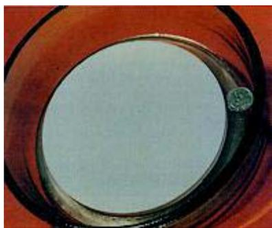
Fig. 5. Opal substance after superficial drying. *Opal substance after superficial drying. It has a diameter of 12.5 cm and a width of 5.5 mm.*
