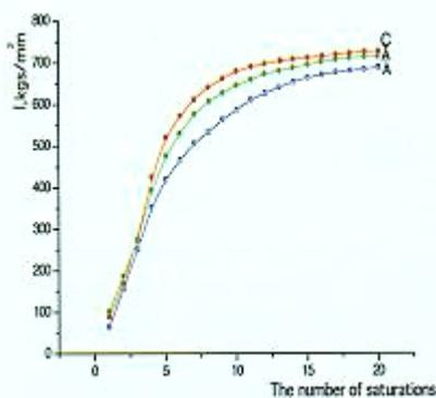
Fig. 7. Dependence of the microhardness of the opal substance on the number of saturations with the silica gels (temperatures of the sintering of the opal substance and the gel: A - 600°C, 400°C; B - 800°C, 800°C; C - 1000°C, 400°C)juh.
