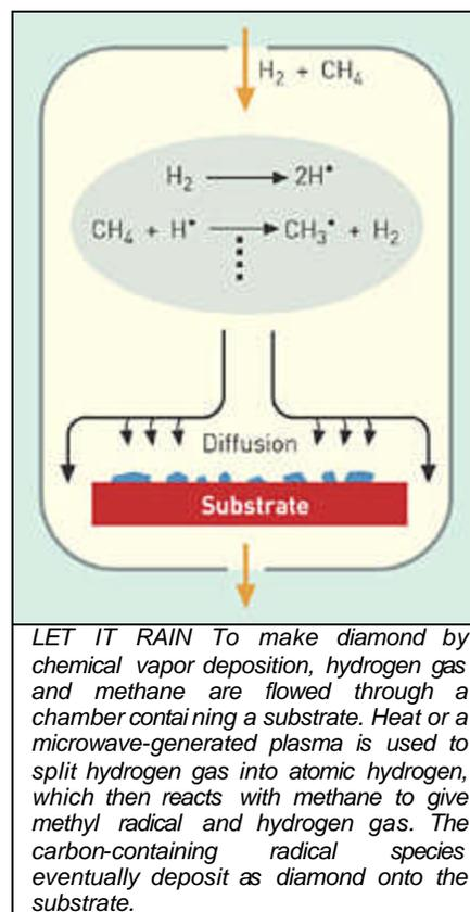
**LET IT RAIN** To make diamond by chemical vapor deposition, hydrogen gas and methane are flowed through a chamber containing a substrate. Heat or a microwave-generated plasma is used to split hydrogen gas into atomic hydrogen, which then reacts with methane to give methyl radical and hydrogen gas. The carbon-containing radical species eventually deposit as diamond onto the substrate.
