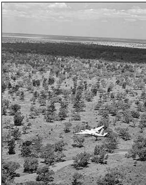
*Plane conducting aeromagnetic survey near Walgett - part of the recently completed 'Discovery 2000' exploration initiative. It is hoped that 'Discovery 2000' and its successor, 'Exploration NSW', will lead to the discovery of commercial petroleum deposits in NSW*
