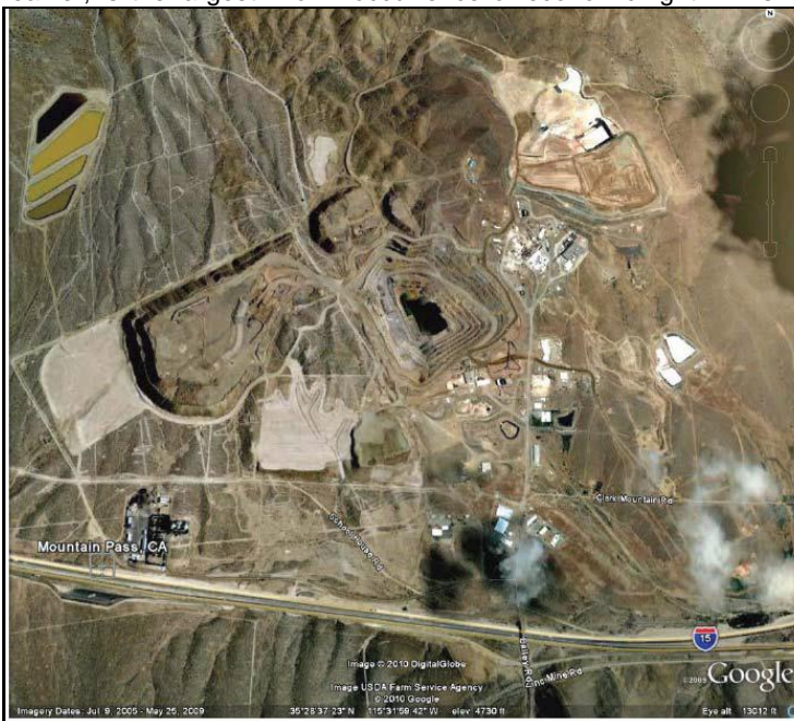
Fig. 6. Google Earth Image of the Mountain Pass mining district, California. Molycorp’s open pit mine – inactive since 2002 – is at the center of this view; the pit covers about 50 acres and is about 400 ft. deep.
