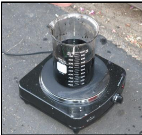
Some Andamooka matrix in a beaker being blackened in a heated acid bath.
